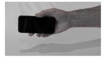
• Fig 1. Simplest option: Holding the mobile device with unsupported arm out-stretched is the simplest way to measure.
